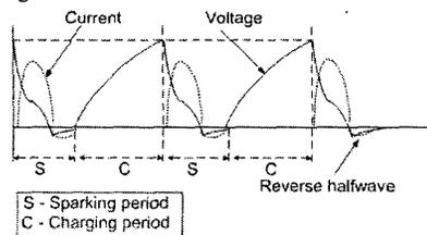
Fig. 3. Voltage and current waveforms for a basic relaxation circuit
