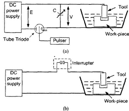
Fig. 4. (a) Pulse generator with a separate pulser; (b) DC interrupter pulse generator
