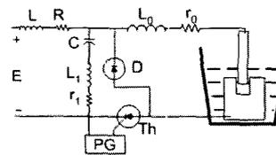
Fig. 8. Thyristorised EDM generator of capacitive type
