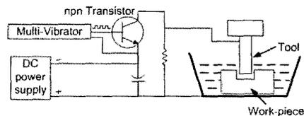
Fig. 5. Typical Transistor switching circuit power supply
