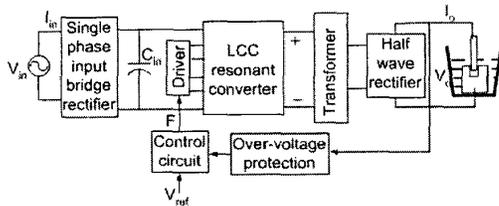
Fig. 14. Basic block diagram of the EDM power supply using a LCC resonant converter
