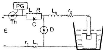
Fig. 11. Thyristorised EDM generator of inductive type
