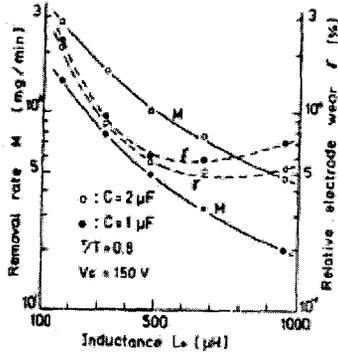
Fig. 10. Effect of induction  $L_0$  on the removal rate for the workpiece M and the relative electrode wear  $\gamma$  in weight [7]
