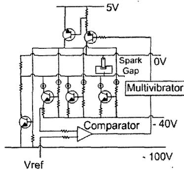
Fig. 13. Circuit diagram of high efficiency supply
