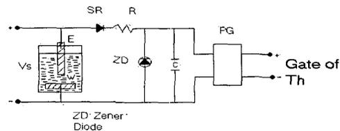
Fig. 9. Preventive Measure for short circuit
