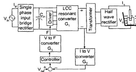
Fig. 15. Basic block diagram of the current controlled EDM power supply system using a LCC resonant inverter
