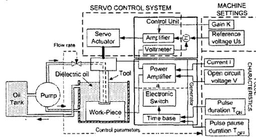
Fig. 1. Schematic layout of basic EDM components
