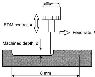
Fig. 5. Surface engraving EDM.
