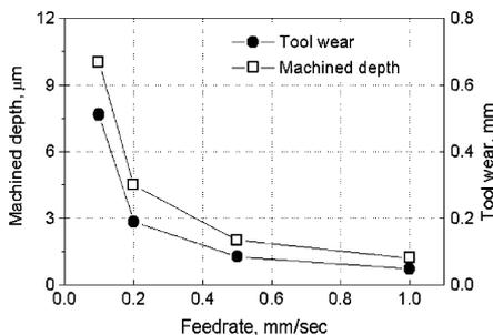
Fig. 8. Influence of feed rate on micro-EDM.
