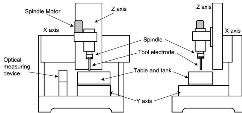
Fig. 2. Structure of desk-top miniature machine tool.
