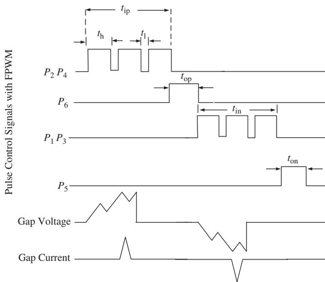
Fig. 3. Timing chart of fixed pulse-width modulated control signals and associated pulse trains of wire-EDM for high-frequency power supply.
