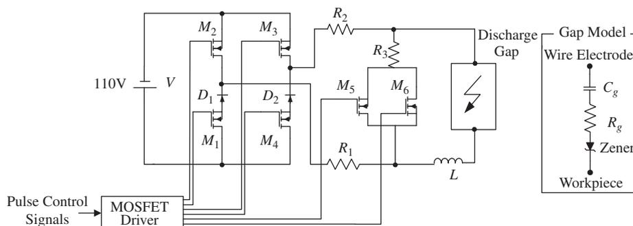
Fig. 2. An anti-electrolysis circuit model for SPICE simulation that uses a RC circuit and a Zener diode for modeling discharge gap.
