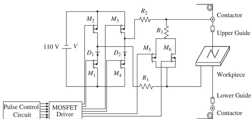
Fig. 1. Circuit diagram of the developed high-frequency power supply for wire-EDM.
