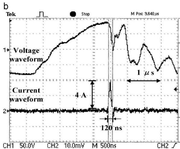
Fig. 4. Pulse waveforms of (a) the developed power supply and (b) original fine-finish power supply.
