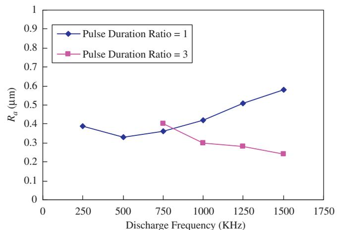
Fig. 5. Effect of discharge frequency on surface roughness of tungsten carbide for different pulse duration ratios. (Brass wire  $\varnothing$ 0.25 mm; wire tension: 1700 gf; wire feed: 5 mm/min; water-resistivity: 125 k $\Omega$ cm; pulse on-time: 240 ns; pulse off-time: 120 ns.)
